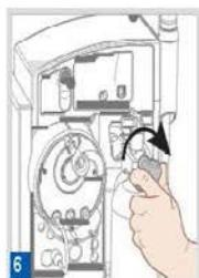
Fully tighten yoke T-handle clockwise.
