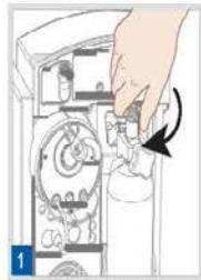
Fully close helium tank valve clockwise.
